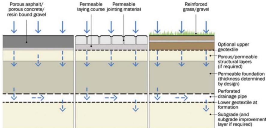
Figure 20.13 Pervious pavement system types: Type B – partial infiltration
