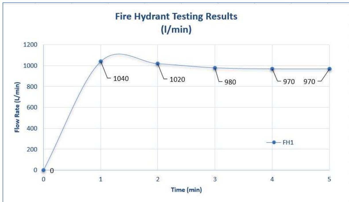
**Figure 3: Fire Hydrant Flow Test Results**
